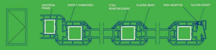
Dimension: Frame - 75mm X 60mm, Shutter - 104mm X 60mm, Mullion - 76mm X 60mm, Glazing Bead - 34mm X 20mm
