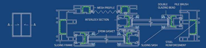
Dimension: Frame - 62mm X 62mm, Shutter - 66mm X 42mm, Interlock - 50mm X 45mm, Glazing Bead - 25mm X 16mm
