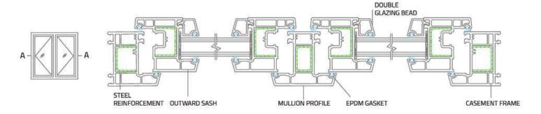
Dimension: Frame - 60mm X 60mm, Shutter - 78mm X 60mm, Mullion - 76mm X 60mm, Glazing Bead - 34mm X 20mm
